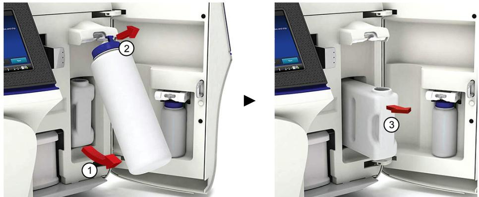
3. Reinstall the empty waste reservoir and a *used* Ion S5™ Wash Solution bottle.
